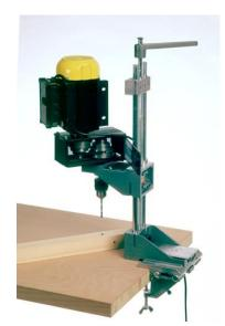
If you like to work in a **vertical position** with the spindle & cranck (**each turn = 4mm way)**, best will be you use **the drilling plate**.
