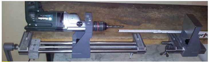
With the extention, you can do horizontal drilling of any length! If you use the crank, you have 4mm advance each turn!
